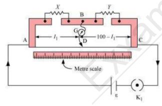
(a) Balance point from end A,  $l_1 = 39.5$  cm Resistance of the resistor  $Y = 12.5 \Omega$
