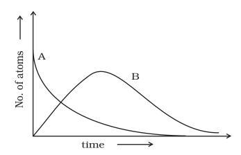
At t=0,  $N_A=N_O$  while  $N_B=0$ . As time increases,  $N_A$  falls off exponentially, the number of atoms of B increases, becomes maximum and finally decays to zero at  $\infty$  (following exponential decay law).
