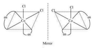
Cis [CoCl<sub>2</sub>(en)<sub>2</sub>]<sup>+</sup>isomer-optically active (Non-superimposable mirror images)
