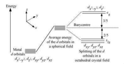
The splitting of the d orbitals in an octahedral field takes palce in such a way that  $d_{x^2-y^2}$ ,  $d_{z^2}$  experience a rise in energy and form the  $e_g$  level, while  $d_{xy}$ ,  $d_{yz}$  and  $d_{zx}$  experience a fall in energy and form the  $t_{2g}$  level.
